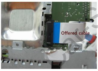
Connect offered FFC cable to subboard.(LCD-IN (BOTTOM))
